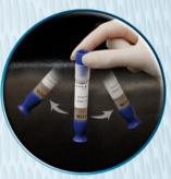
4 → Shake energetically the collecting vial to homogenize the solution before testina.
