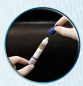
5 → Unscrew the blue testing cap at the bottom of the collecting vial.
